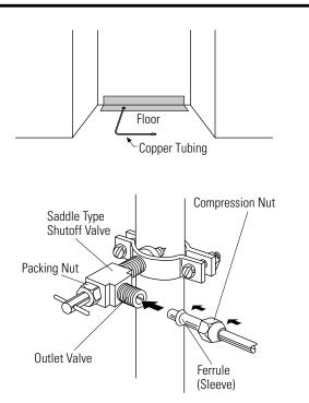
**NOTE:** Saddle type shut-off valves are included in many water supply kits. Before purchasing, make sure a saddle type valve complies with your local plumbing codes.
